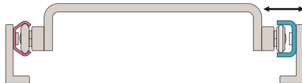
T and U rail allows for misalignment
