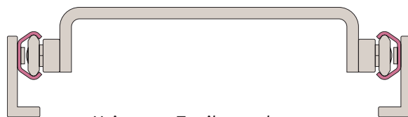
Using two T rails good set-up accuracy is required
