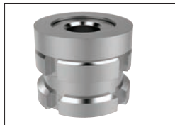
62040 - Designed for applications requiring both height adjustment (from 4 to 14mm) and precise adjustment of non-parallel surfaces, with a maximum angle of tilt 4°.
